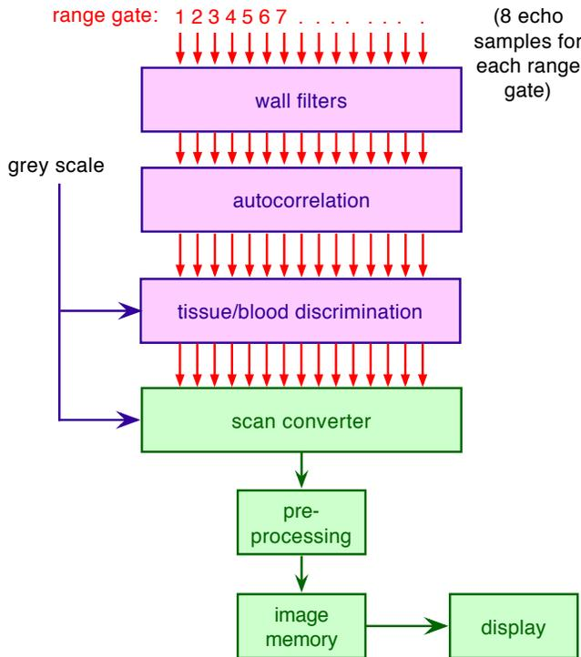
Figure 7.29 Block diagram showing in more detail the colour Doppler processing and image formation.
