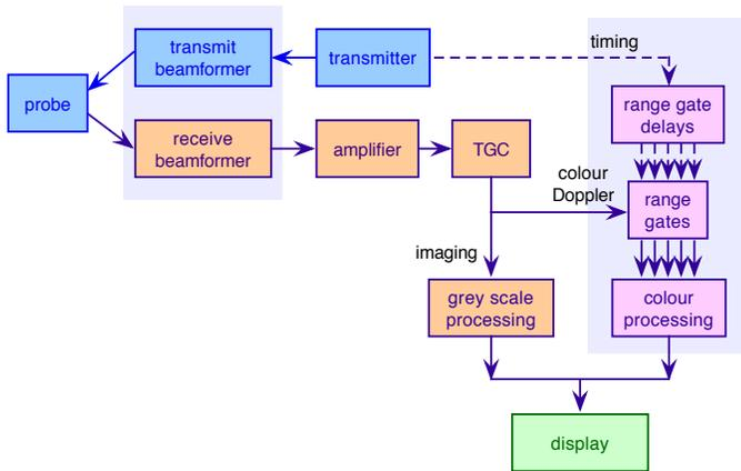
Figure 7.26 Block diagram showing colour Doppler processing incorporated into a grey scale imaging machine.
